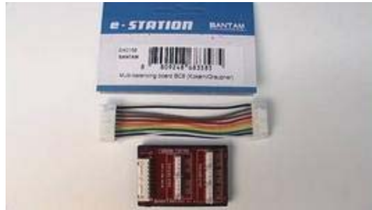
This is a typical multiple battery charging connection board.
